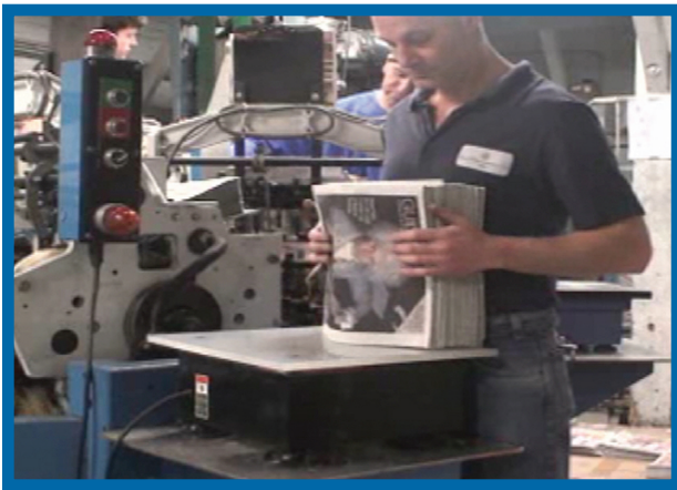
Westerly Sun (Westerly, RI) employee using PJT-100 to align inserts.
